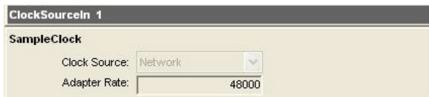
Figure 22. Clock Source information for CobraNet devices as seen in ASIControl.
