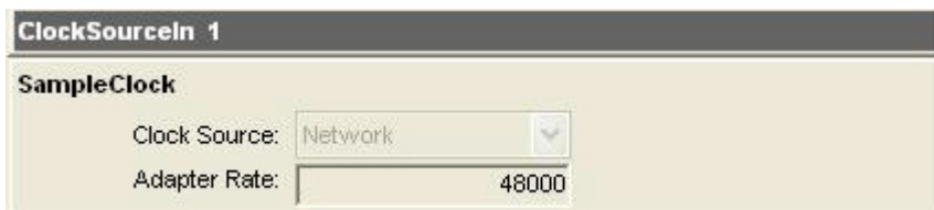
Figure 21. Clock source information for CobraNet devices as seen in ASIControl
