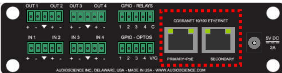
There are two RJ-45 Ethernet jacks on the rear of the unit. If a redundant CobraNet network is not being used then plug a network cable into the PRIMARY jack. If a redundant network is being used then plug a second network cable into the SECONDARY jack. (See [http://cobranet.info/support/design/switched\\_networks](http://cobranet.info/support/design/switched_networks) for information on redundant networks.)
