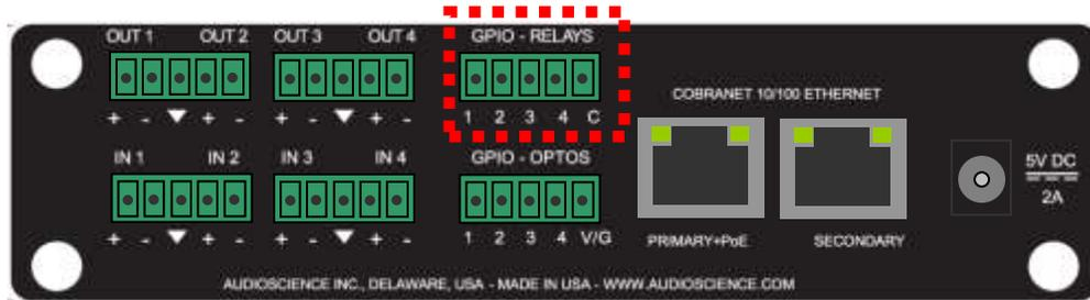
Each outputs consists of a normally open relay with one side connected to a common pin (C). The current through each relay should be limited to 500mA.
