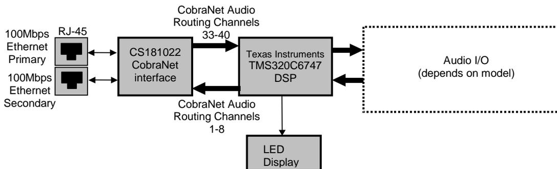
Figure 1. Hono Mini CobraNet Mini interface block diagram
