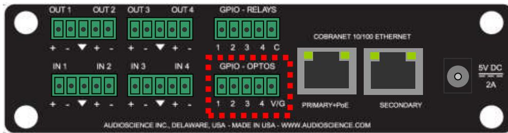
The voltage powering the LED in the opto-isolator may either be supplied from an external source through the V/G pin or may be powered from the Hono Mini's internal +5V supply. The opto-isolator voltage is software selectable using ASIControl and the setting is stored in the units non-volatile memory,
