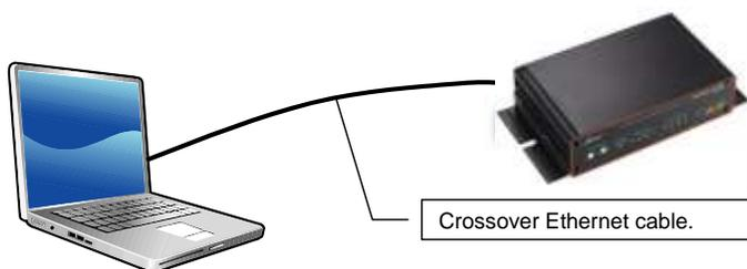
**Figure 14. Laptop to Hono Mini CobraNet interface connection**
