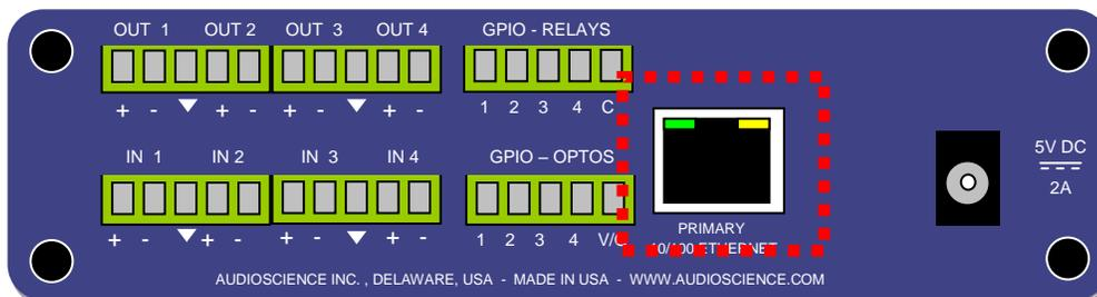
A CAT-5 or better (CAT-5e, CAT-6 etc) network cable is required for 100baseT Ethernet operation. The cable length between the Hono Mini interface and a network switch should not exceed 100 meters (328 feet)
