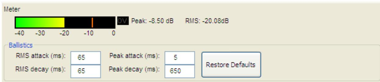
Figure 6. A stereo peak meter display; RMS is green and peak is yellow
