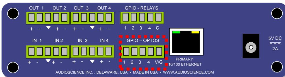
The voltage powering the LED in the opto-isolator may either be supplied from an external source through the V/G pin or may be powered from the Hono Mini's internal +5V supply. The opto-isolator voltage is software selectable using ASiControl and the setting is stored in the units non-volatile memory,
