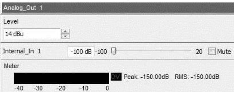
Clicking on Analog\_Out 1 in the topology pane of ASIControl will show a list of volumes in the node view pane. At left is an image of the Level section, the first volume control and the Meter control shown in the node pane. The meter is found after the full list of volumes (the Hono Mini AVB interface incorporates AudioScience’s anything to anywhere’ mixing).
