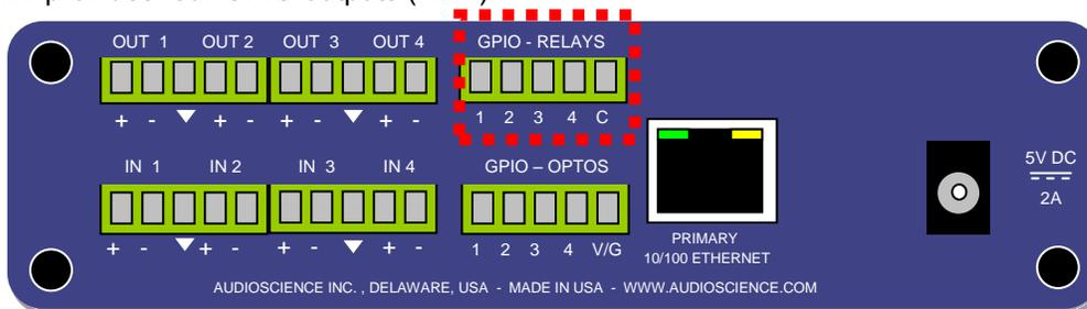
Each outputs consists of a normally open relay with one side connected to a common pin (C). The current through each relay should be limited to 500mA.
