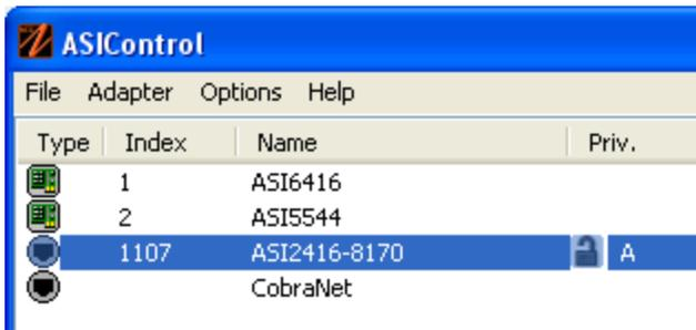
By default, if a password has not been set, the adapter operates as if there is no active password. Any user has complete access to all the device functionality.
