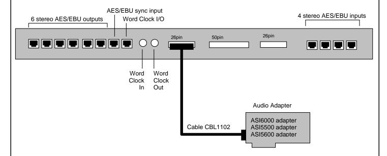
**NOTE**: On ASI6518 or ASI6618 sound cards, AES inputs 3 and 4 can be assigned as outputs 7 and 8. This allows one BOB1025 to be used; it will then have 8 AES/EBU 'outputs'. Please refer to the ASI6518/ASI6618 datasheet for further information on how to set this up.
