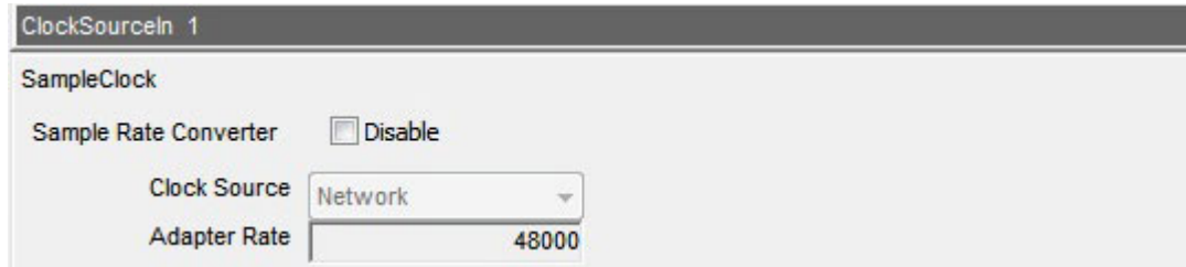
Figure 10 Clock Source information for AudioScience Con\braNet sound cards as seen in ASIControl
